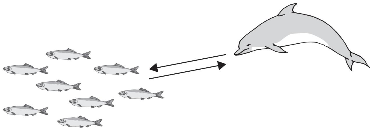
The dolphin sends out an ultrasound pulse and the echo returns 0.04 seconds later. Ultrasound travels at 1500 m/s in water.
