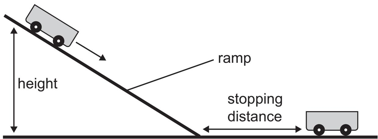
He changed the height of the ramp and measured how far the trolley travelled from the end of the ramp.
