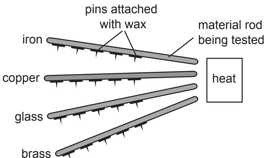
The number of pins still attached to each rod was recorded after 1, 3 and 5 minutes. The results are shown below.
