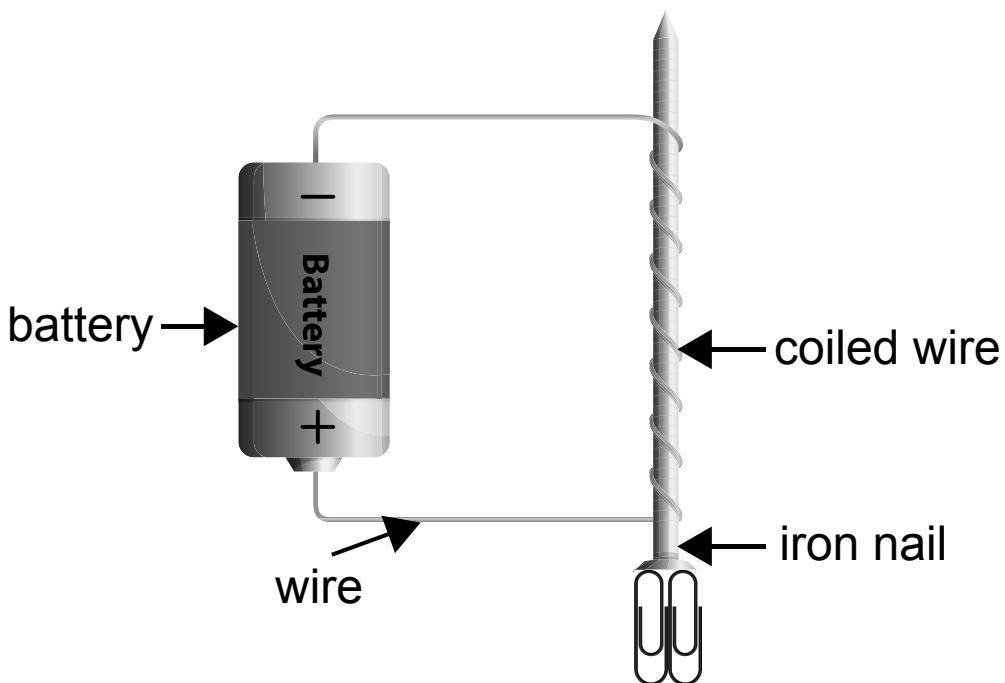
A student wanted to see how the number of paper clips the magnet was able to pick up depended on the size of the current passing through the wire. The current was changed to different values and the number of paper clips counted each time.
