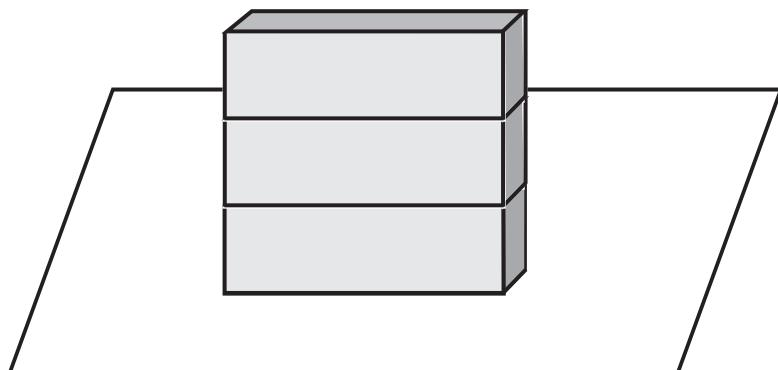
The weight of each block is 20 N and the area in contact with the surface is 1.5 m<sup>2</sup>.
