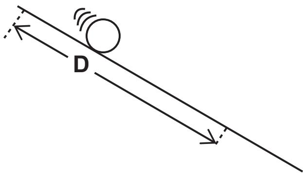
The time taken for the ball to travel a distance D was measured on three occasions and the average time T was recorded. This was then repeated for different distances.
