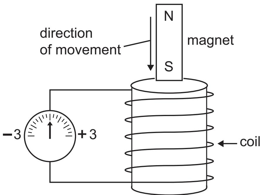
(a) When a pupil moves the magnet into the coil the needle on the ammeter moves to +2 and then returns to zero.
