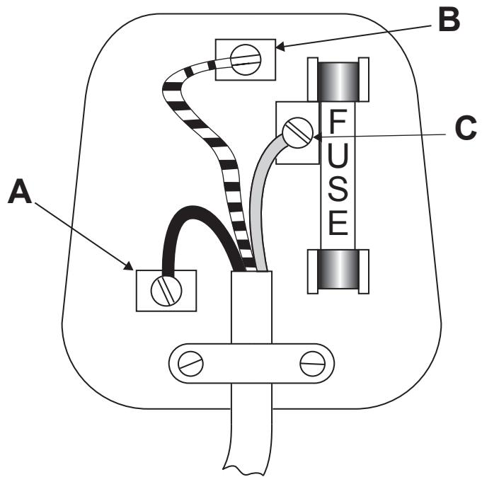
**(i)** Which pin A, B or C is the earth pin? [1]
