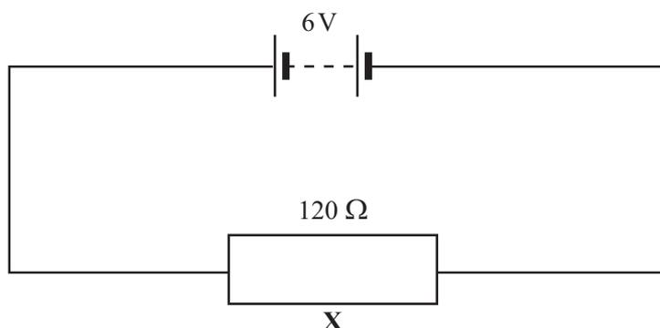
**10.1** The battery consists of 1.5 V cells connected in series. The number of cells needed is . . . . .
