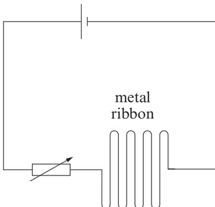
(a) (i) **Add meters to the circuit** that allow you to calculate the resistance of the metal ribbon. [2]
