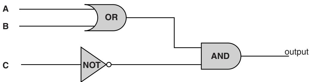
(a) Complete the truth table for the logic circuit.
