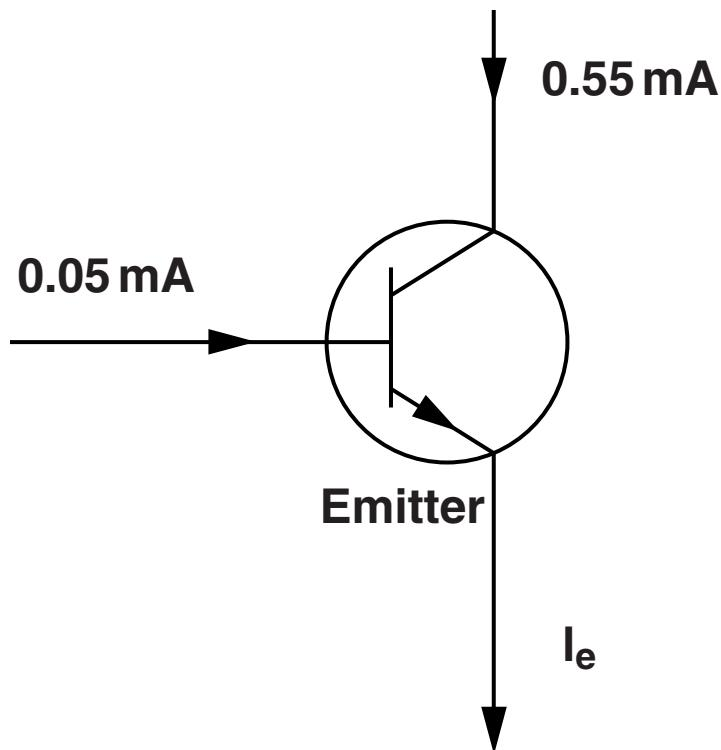
Calculate the current flowing from the emitter,  $I_e$ .
