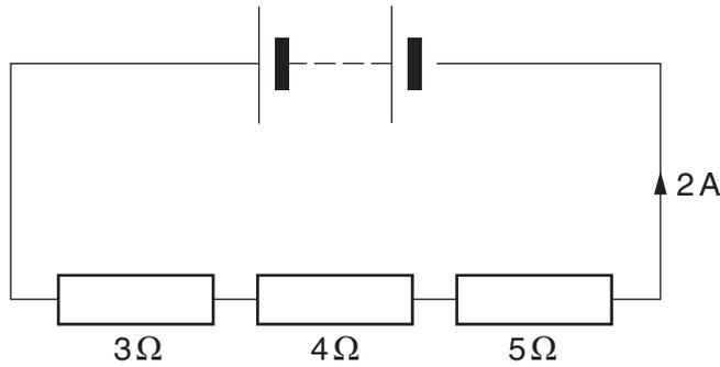
(a) What is the voltage across the  $3\ \Omega$  resistor?
