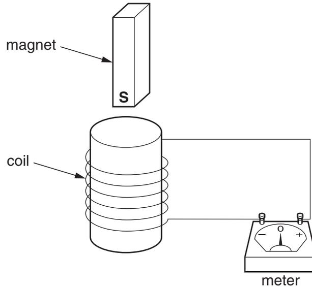
Experiments with this apparatus can show how the electricity is generated.
