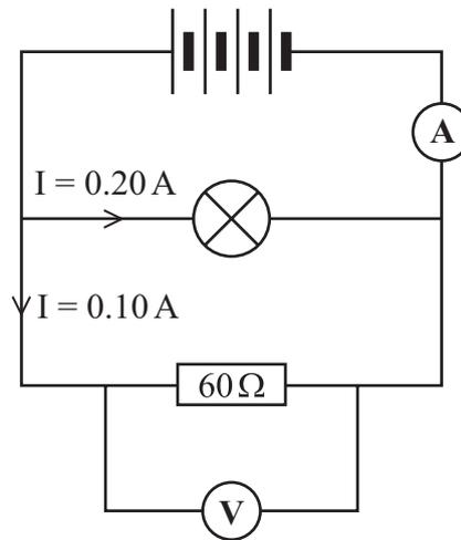
4 (a) Each cell provides a potential difference of 1.5 volts.
