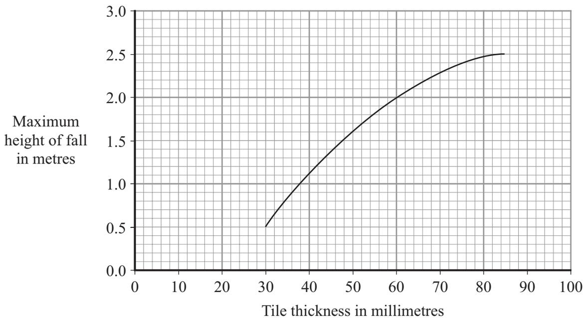
6 (a) (i) Describe how the maximum height of fall relates to the thickness of the rubber safety tile.
