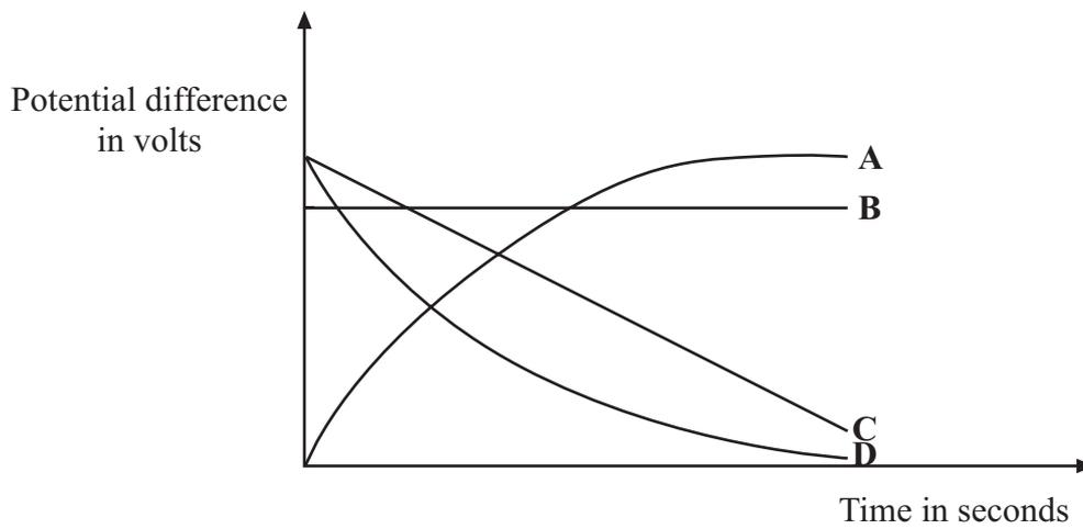
**10.2** The variable resistor is adjusted. It now takes a shorter time to charge the capacitor.
