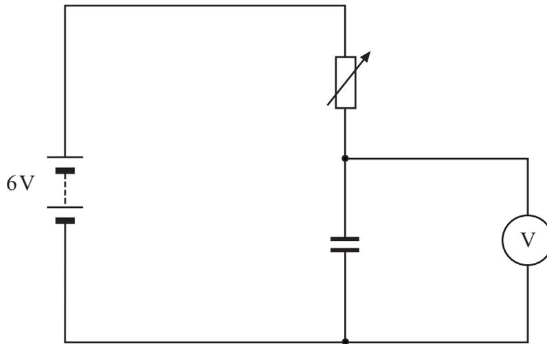
**10.1** Which graph line shows the change in potential difference across the capacitor as it is being charged?
