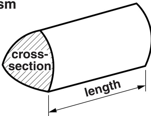
$$\text{Volume of prism} = (\text{area of cross-section}) \times \text{length}$$
