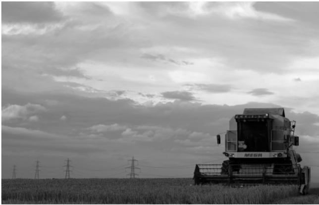
The barley would be used to produce malt, used in beer and Maltesers. The huge machine, with just one driver, replaced three smaller combine harvesters. It can unload grain into a trailer whilst on the move. This cuts down the time needed to harvest a field and the amount of crop wasted by inefficient harvesting.
