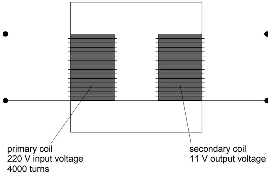
(a) Calculate the number of turns in the secondary coil.
