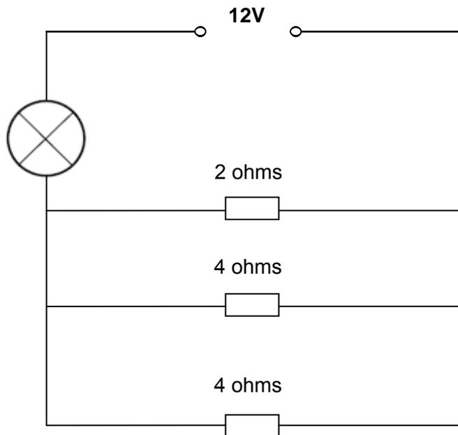
Calculate the **total resistance** of the three resistors.
