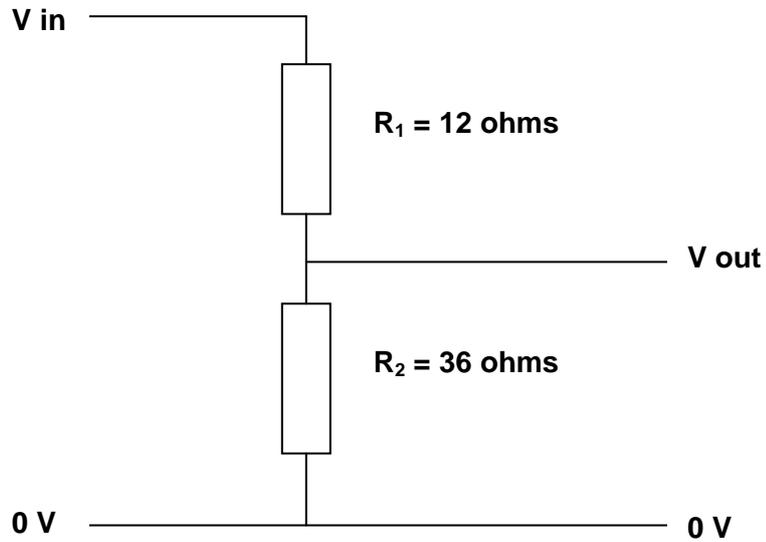
The **input** voltage =  $5\text{ V}$ .
