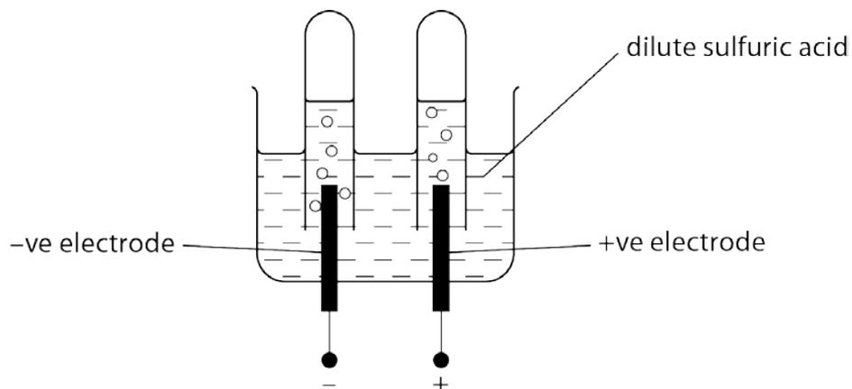
(a) Bubbles of gas are made at both electrodes.
