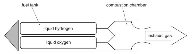
The hydrogen particles react violently with the oxygen particles in the combustion chamber.
