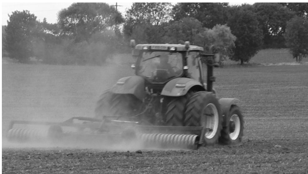
The farmer has fitted double wheels to the tractor to reduce soil compaction.
