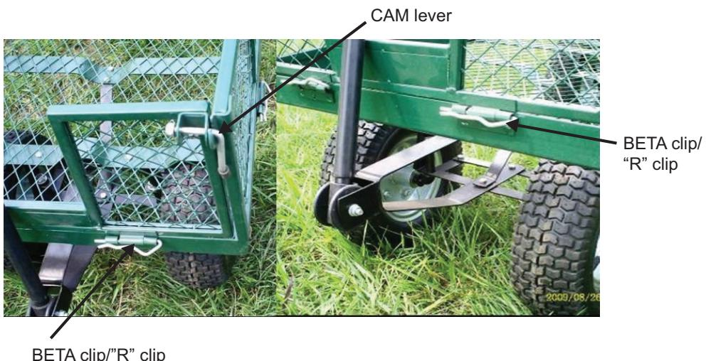
When the CAM lever is lifted the CAM lifts the handle out of the bracket. The sides are secured on using beta pins and hinges which allow them to fold down and detach from the trolley. There is a hinge on the side and on the frame of the trolley. When the two beta clips are removed and the CAM lever is lifted out of the bracket, the sides can be detached.
