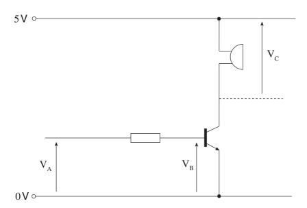
The transistor is just saturated when the input voltage  $\boldsymbol{V}_{\boldsymbol{A}}$  is 2.5 V.
