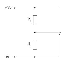
$$V_{\text{OUT}} = \frac{R_2}{R_1 + R_2} \times V_{\text{S}}$$
