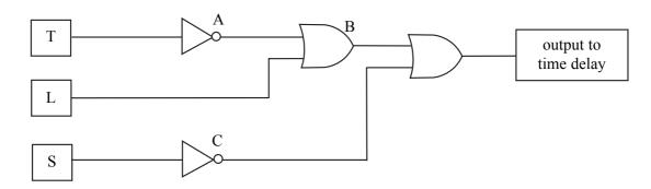
(a) A low voltage output is required to trigger the time delay. Complete the truth table below for the network of gates.
