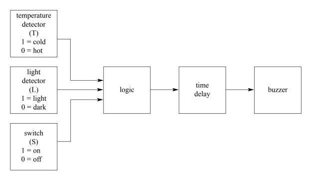
This network of gates is used for the logic.
