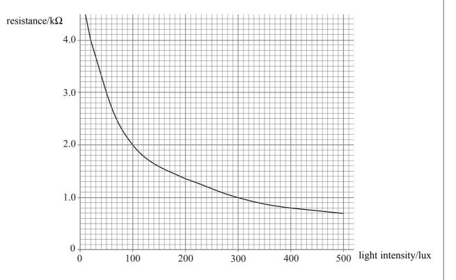
(i) In a test the student finds that the light intensity is 50 lux when the beam is broken. From the graph, find the resistance of the light dependent resistor at 50 lux.
