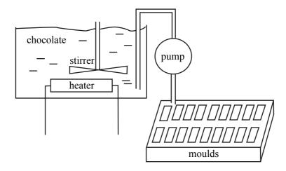
The heater, stirrer and pump are controlled electronically by this system.
