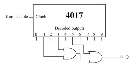
Complete the timing diagram below to show the output from Q as pulses are fed into the clock input.
