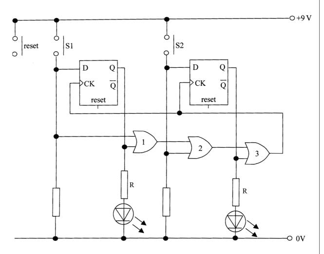
(a) On the diagram above add **one** extra component and the connecting wires which are needed to allow the referee to reset the circuit.
