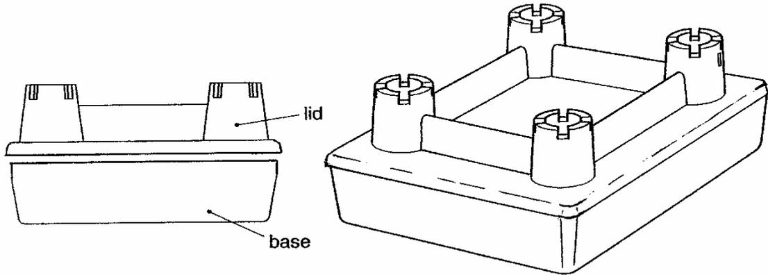
(a) Both parts of the box are vacuum formed in 3mm thick High Impact Polystyrene (HIPS).
