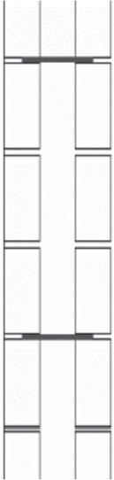
Cavity walls were the first development to prevent the spread of damp into the inside of buildings. These walls were constructed from two skins of brick or block joined together by twisted galvanized steel wall ties. The twist was constructed into the wall ties so that any moisture which tried to move across the cavity would drop off.
