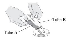
**Step 2** Mix the liquids to make the glue. Put a thin layer of the glue onto each of the surfaces to be joined.
