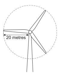
**4 (a)** The blades of the turbine are 20 metres long. On average, 15 000 kg of air, moving at a speed of 12 m/s, hit the blades every second.
