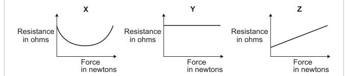
Which of the sensors, X, Y or Z, would be the best one to use as a force sensor?
