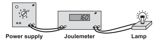
The student set the joulemeter to zero, and then switched on the power supply.
