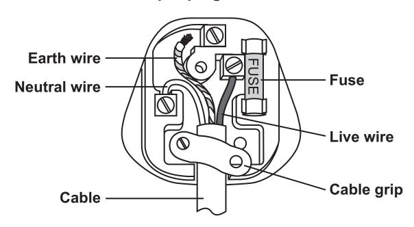
5 (a) (i) What TWO changes need to be made so that the plug is wired correctly? [2 marks]
