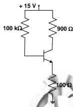
Which one of the following correctly represents the load line (collector current I<sub>C</sub> with respect to collector-emitter voltage V<sub>CE</sub>) and Q-point of this circuit?
