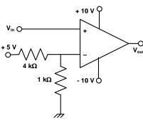
Which one of the following correctly represents the output  $V_{out}$  corresponding to the input  $V_{m}$ ?
