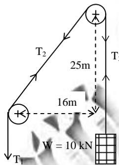
The tensions  $T_1$  and  $T_2$  respectively in kN are
