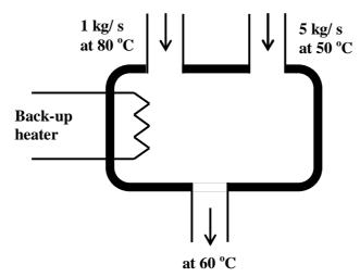
There is no accumulation of water in the tank. A back-up heater is provided to ensure a constant outflow temperature of water at 60 °C from the tank under steady state. What is the required capacity of the back-up heater to the nearest kW?
