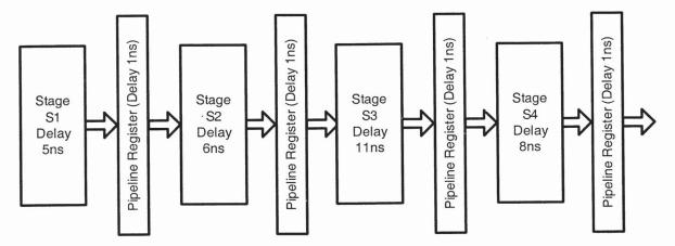
What is the approximate speed up of the pipeline in steady state under ideal conditions when compared to the corresponding non-pipeline implementation?
