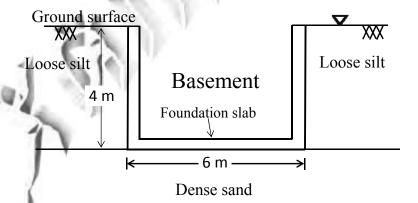
Using factor of safety = 3, the net safe bearing capacity (in  $kN/m^2$ ) of the foundation is: O.52
