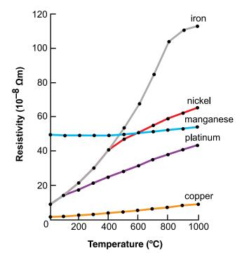
Which metal is the poorest conductor at 400 °C?
