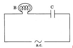
How will the glow of the bulb be affected on introducing a dielectric slab between the plates of the capacitor? Give reasons in support of your answer.
