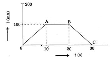
Calculate the value of E.C.E. of copper in terms of the mass, m, deposited.
