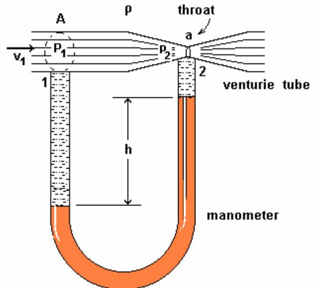
Using Bernoulli's theorem at points '1' and '2' which are at the same elevation,
