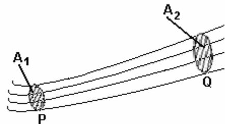
$$\frac{dm}{dt} = \rho_1 A_1 v_1 = \rho_2 A_2 v_2$$
