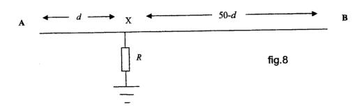
In order to locate the fault, the following procedure is used. A potential difference of 200 V is applied to end A of the cable. End B is insulated from the ground, and it is measured to be at a potential of 40 V.
