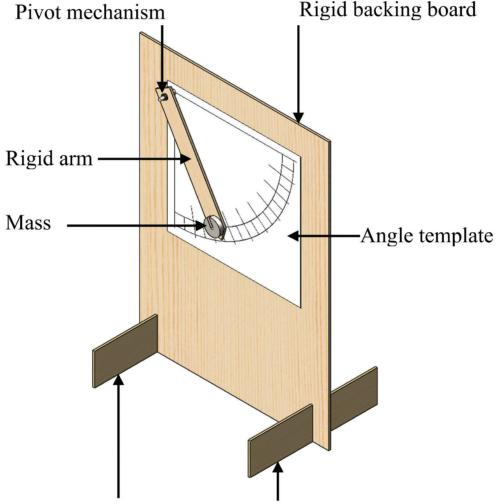
Supports slotted into rigid backing board
