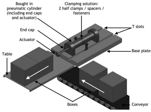
Size of base plate: Thickness - 20mm; Length - 250mm; Width - 150mm Material: Aluminium
