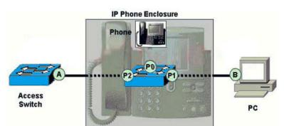
If a 7960 IP phone sends voice media frames towards the access switch, how will these frames be observed at point A
