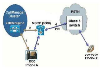
Assume that the gateway is a 6608 blade configured as a gateway and running MGCP; Call Manager runs version 3.1, and that a call is made from phone A to phone X. All IP streaming is G.711. Each of the logical links represented carries certain types of traffic. On which links can q.931 traffic be seen?
