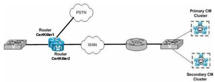
Should a WAN failure occur while the primary router, Router Certkiller 1 is in use, Router Certkiller 1 should switch to SRST mode to preserve telephony functions. However, if Router Certkiller 1 also fails, the HSRP backup router, Router Certkiller 2, must become the active router for the branch office and must take over SRST and routing functions for the branch office.
