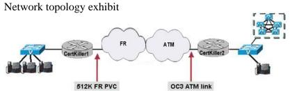
Consider the WAN network in the picture shown. The speed of the FR PVC connecting Router Certkiller 1 to the FR network is such that fragmentation is required when a voice call is present across the WAN. The speed of the ATM PVC connecting Router Certkiller 2 is high enough not to require fragmentation. Which technologies are involved in the QoS solution needed for this scenario.
