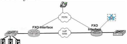
You want to implement Caller ID for calls from PSTN to the IP Phones. Analog trunks are equipped to the PSTN from both the GWs. The PSTN CO switch is capable of delivering Caller ID on the connection to the Cisco voice GW. The Cisco voice gateway is using a VIC-2FXO-M1 card. What would be the correct voice GW design?
