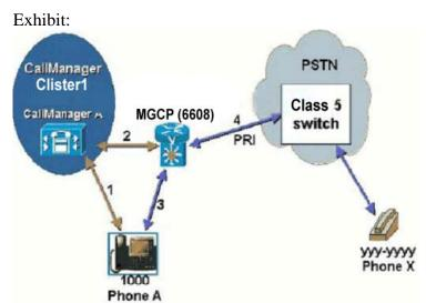
Assume that the gateway is a 6608 blade configured as a gateway and running MGCP; Call Manager runs version 3.1, and that a call is made from phone A to phone X. All IP streaming is G.711. Each of the logical links represented carries certain types of traffic. On which links can RTP traffic be seen?
