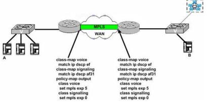
The LAN switches (and any other equipment in the cloud) do not mark or remark the packets.
