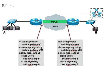
Consider the QoS configuration in the picture shown for a VoIP call across an MPLS network. If IP Phone A calls IP Phone B, how will voice and signaling packets be marked by the time they arrive at the IP Phone B? NOTE: Assume the LAN switches (and any other equipment in the cloud) do not mark or remark the packets, and the complete MPLS router QoS configuration is shown in the picture.
