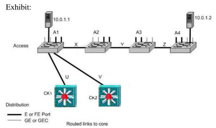
The diagram shows a wiring closet stack of four L2 switches A1, A2, A3, and A4. A1, A2, A3 and A4 are connected in series. Switch A1 is the root switch and connects to CK1 and CK2. There are no loops in the wiring closet VLAN (=subnet). The architect wants to remove X, Y and Z, and connect A1 directly to A2, A3, and A4 in s star. Is this a good idea?
