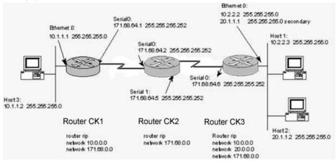
With RIP running, what command would be used to set the default route on Router CK2 to 171.68.64.6 (Router CK3)?
