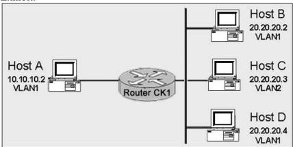
Host D sends a frame to Host B at the same time that Host B sends a frame to Host D. Bridging is enabled on Router CK1, and the two frames collide into each other. Select the best explanation of why Host B will or will not receive the original frame from Host D:
