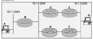
In this diagram, Host G is attempting to send a packet to Host A through Router E. All routers are
