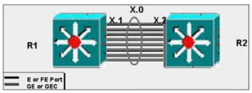
L3 switches R1 and R2 are in the backbone of the network. They are connected by a routed EtherChannel bundle consisting of eight Gigabit Ethernet ports. The routed link is represented as subnet X.0 in the diagram. Since X.0 is routed, it is not a VLAN trunk. How can spanning tree loops be prevented in the backbone of this network?
