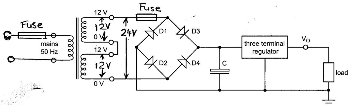
It was acceptable to place a fuse in either the primary or secondary part of the transformer.
