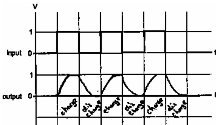
A variety of waveforms were accepted, including those that were similar to the input. Many students sketched an inverted square wave, which was not accepted.
