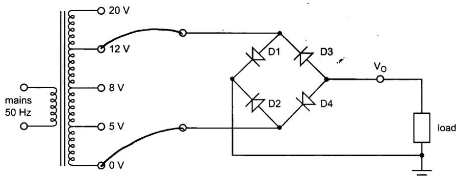
This question required students to make some rough determinations about the stated RMS voltages on the multiple tapped transformer when converted to the possible peak voltages. Both the 0 V and the 12 V tap had to be connected to the bridge rectifier. The following mathematical solution proves the 0 V and 12 V connections are correct.
