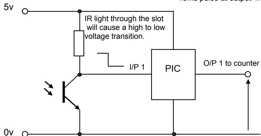
PIC will detect the change in voltage level and produce a 10ms pulse at output 1.
