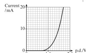
(ii) Comment on the resistance of the LED at voltages below 1.0 V. Calculations are not required.
