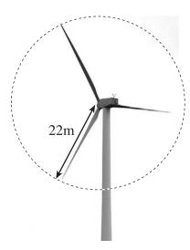
(i) The volume of air passing through the blades every second can be calculated by considering a cylinder of air incident on the blades. Show that the volume of air passing through the blades in one second is approximately 21000 m<sup>3</sup> s<sup>-1</sup>, when the wind speed is 14 m s<sup>-1</sup>.
