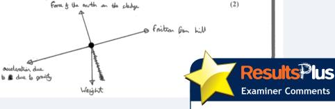
This has the three correct forces and all in the correct direction. There is an additional arrow, labelled acceleration, which should not be added to a free body force diagram. In addition, without details of the speed, it isn't possible to determine whether it is accelerating or travelling at constant velocity.
