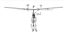
(i) Add labelled arrows to the diagram to show the forces acting on the cable at the point P.
