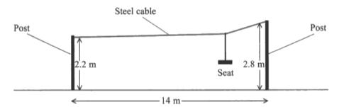
A child sits on the seat which moves on runners along the cable from the high end to the lower end.
