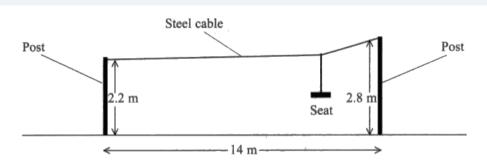
A child sits on the seat which moves on runners along the cable from the high end to the lower end.
