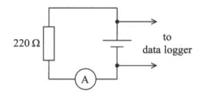
The student proposes to use a data logger to monitor the terminal potential difference (p.d.) of the cell over a period of time.
