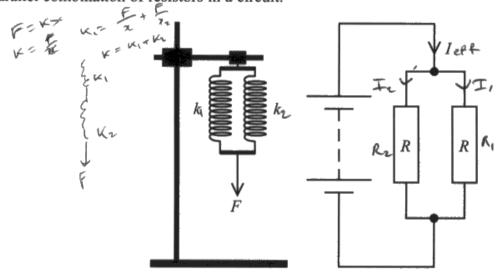
(a) Derive an expression for the effective resistance  $R_{eff}$  of two resistors  $R_1$  and  $R_2$  connected in parallel in a circuit.
