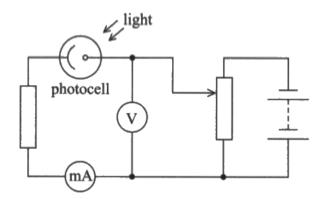
The student illuminates the photocell with light of known frequency f. A current is produced in the circuit due to the emitted electrons. He adjusts the potential difference, using a potential divider, until the reading on the milliammeter is zero and records the corresponding reading  $V_s$  on the voltmeter. He repeats this procedure for other frequencies of light.
