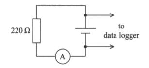
The student proposes to use a data logger to monitor the terminal potential difference (p.d.) of the cell over a period of time.
