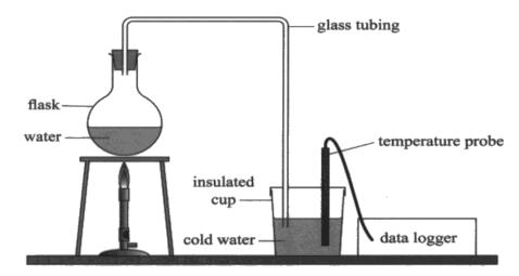
The water in the flask was heated and steam was forced out of the flask and through the glass tubing into the cold water in the insulated cup. The steam condensed as it passed into the cold water.
