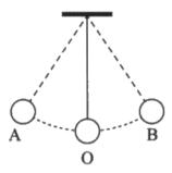
The student releases the pendulum at A and simultaneously starts the stopwatch. She measures the time taken for 5 oscillations and divides the value by 5. She repeats the procedure twice and calculates a mean time period.
