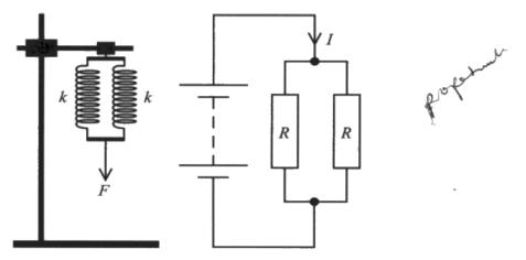
(a) Derive an expression for the effective resistance  $R_{eff}$  of two resistors  $R_1$  and  $R_2$  connected in parallel in a circuit.
