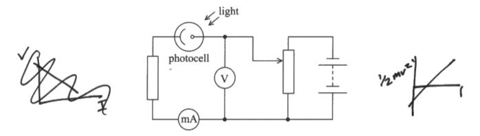
The student illuminates the photocell with light of known frequency f. A current is produced in the circuit due to the emitted electrons. He adjusts the potential difference, using a potential divider, until the reading on the milliammeter is zero and records the corresponding reading  $V_s$  on the voltmeter. He repeats this procedure for other frequencies of light.  $hf = \mathcal{D} + \frac{1}{2}mr^2$
