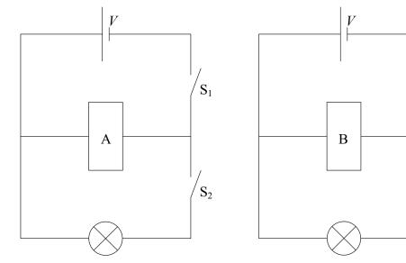
The switches  $S_1$  are closed for a few seconds and then opened. The switches  $S_2$  are then closed. The lamp connected to box A is seen to light for longer than that connected to box B.
