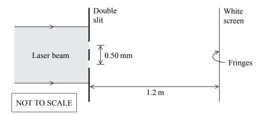
The light from the slits superposes forming an interference pattern on the screen. For this arrangement the measured distance across 40 fringes is 49.6 mm.
