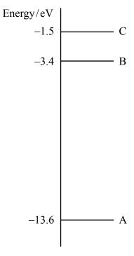
(a) Excited hydrogen atoms can emit light of wavelength 656 nm. By means of a suitable calculation, determine which transition between energy levels is responsible for this emission.
