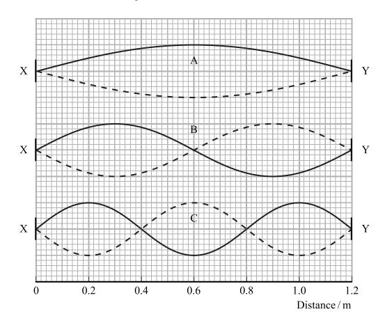
(i) Wave A has a frequency of 110 Hz.
