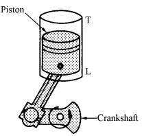
As the crankshaft rotates through  $360^\circ$ , the top of the piston moves from L to T and back to L. The distance LT is 8.6 cm and the crankshaft rotates at 6000 revolutions per minute.
