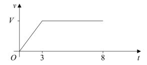
(a) (i) During the first 3 seconds the bus accelerates at  $0.8 \,\mathrm{m\,s^{-2}}$ .
