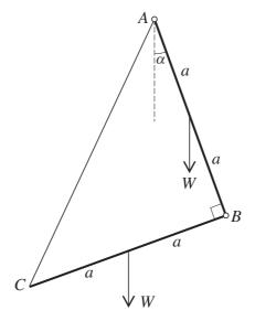
Two uniform rods, AB and BC, each have length 2a and weight W. They are smoothly jointed at B, and A is attached to a smooth fixed pivot. A light inextensible string of length  $(2\sqrt{2})a$  joins A to C so that angle  $ABC = 90^{\circ}$ . The system hangs in equilibrium, with AB making an angle  $\alpha$  with the vertical (see diagram). By taking moments about A for the system, or otherwise, show that  $\alpha = 18.4^{\circ}$ , correct to the nearest  $0.1^{\circ}$ .
