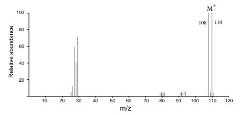
There are **two peaks for the molecular ion**, one for the molecule containing the isotope <sup>79</sup>Br and the other for the one with the <sup>81</sup>Br isotope. **Because the two isotopes are of similar abundance**, **the peaks are of similar height**.
