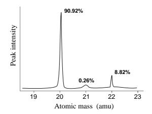
Fig. mass spectrum of the three neon isotopes
